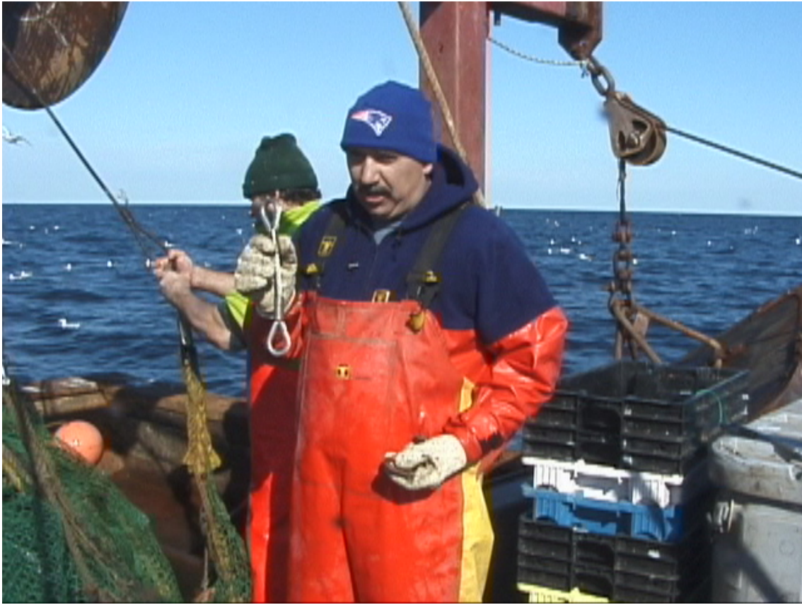
Figure 3: Extension piece added during at sea modification of the sweepless RFT to raise the footrope off the seafloor.
